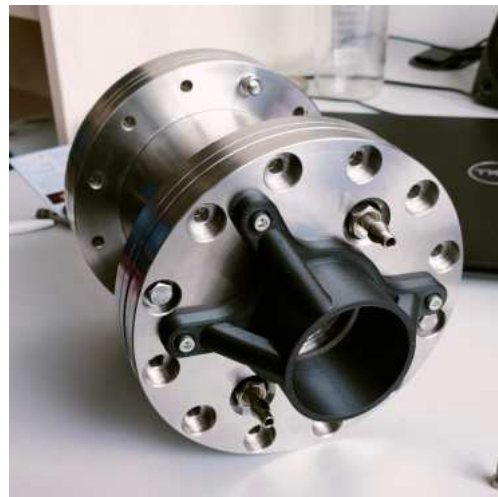
(c) Closed test cell with the PMT holder mounted at the front
