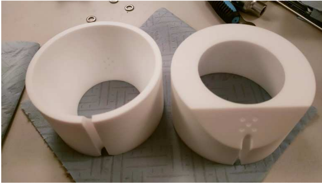
Fig. 4.9.: Picture of the two insets creating a paraboloidal shape with additional cut outs.
