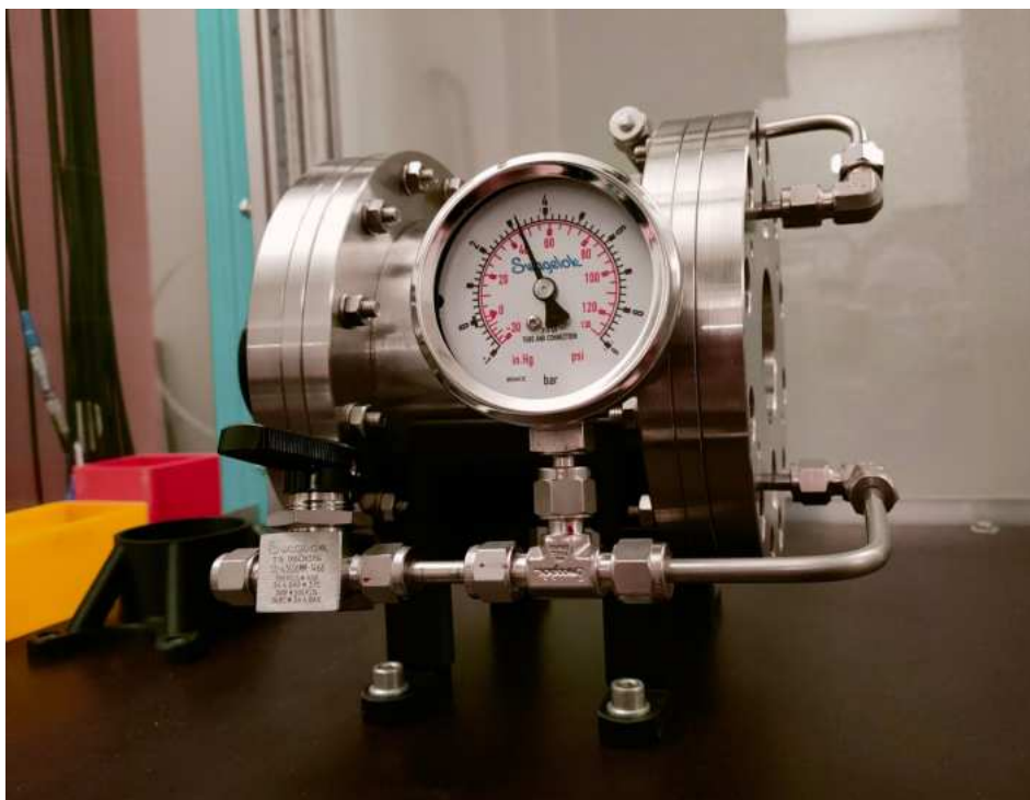
Fig. 5.2.: Picture of the cell mounted vertically on the rack. On the right side of the cell, at the two pipe connectors, the piping is installed up to the two valves
