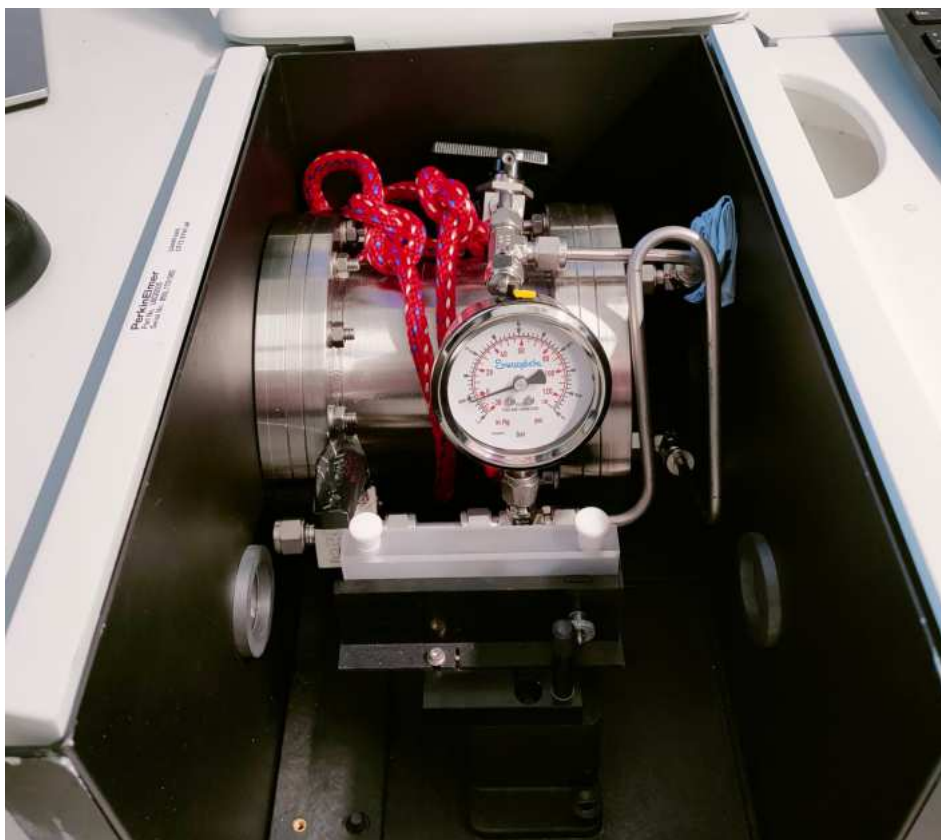
Fig. 5.4.: View inside the spectrometer with the test cell tightly fitting in the back light path and a cuvette in the front light path. The red rope around the test cell is installed in order to lift the cell in and out of the spectrometer
