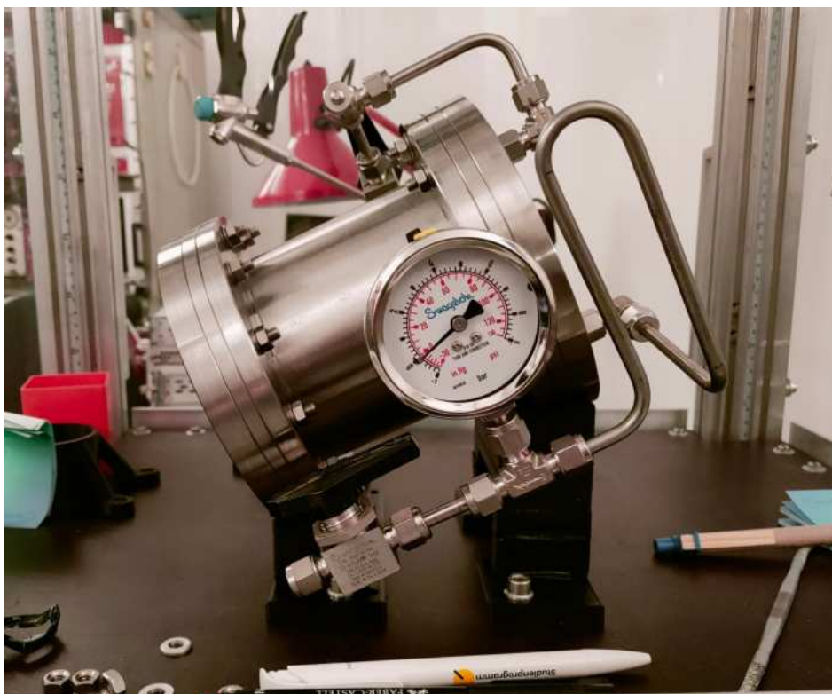
Fig. 5.3.: Picture of the test cell mounted on the tiled holder, which is used for the gas loading of the cell. The pipe connected at the bottom is updated to the first design to avoid liquid flowing back into the filling system.
