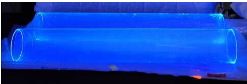
Fig. 4.1.: Image of an inner tube of the WOM illuminated by an UV lamp
