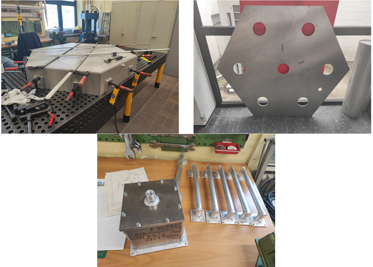
Figure 6.3: Assembly and welding of veto system components.
