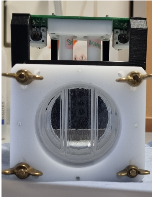
Figure 4.4: Look into the LS cavity through the PMT hole. The cavity is filled with transparent LS, Bis-MSB coated bubo-fibres are inserted. Reflective foil is glued to the opposite glass window. The black holding structure holds the board where the SiPMs are mounted to. The fibre ends are connected to the SiPMs via the white fixing structure.
